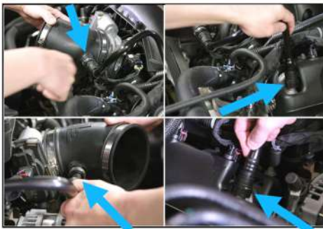
23. Connect both PCV/TUBES onto INLET/DUCT and valve cover.
