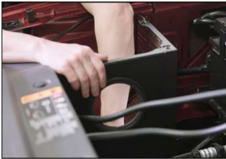
20. Install performance AIR INDUCTION HOUSING into vehicle making sure the rubber mounting grommets slide into the grommets on vehicle.
