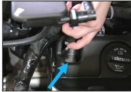
5. Unclip PCV fitting from valve cover.
