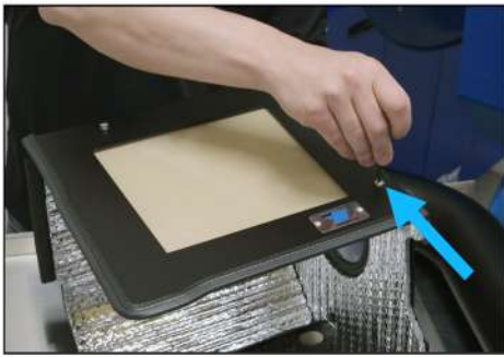
17. Remove COVER from the performance AIR INDUCTION HOUSING with a 3mm allen wrench.
