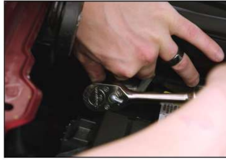
30. Reconnect battery terminal with 10mm socket and ratchet.
