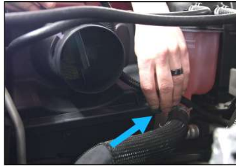
8. Remove MAF wire harness from the AIR INDUCTION HOUSING.
