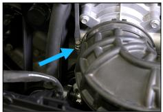
6. Loosen worm clamp on throttle body using 8mm nut driver.
