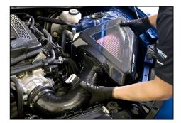
13. Lubrication of the mounting grommets before seating the air induction housing is suggested for easier installation. Gently push the MAF/tube into the hump coupler, and lower the air induction housing into its position. Seat it securely in the three mounting grommets. It should line up perfectly and have a snug fit in your engine bay.
