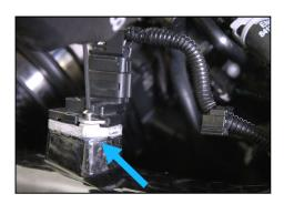
16. Install the MAF sensor into the housing. Tighten the 2 button head screws with the 2.5 mm allen wrench
