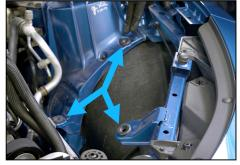
9. Reinstall any of the 3 OEM grommets that may have stayed attached to the factory air induction housing assembly.
