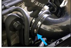
14. Tighten the screws on the hump coupler nearest the intake tube. Torque specs 5.1 +/-0.5Nm
