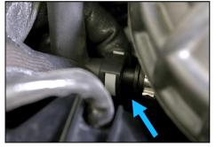
7. Pinch the grey clips to remove the quick disconnect tube from the top of the PCV port.
