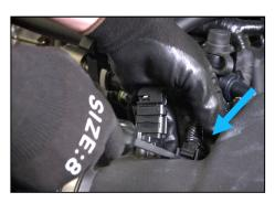
3. Detach the MAF sensor cable clip gently with screwdriver.
