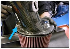
10. Place the filter on a table with the open side up. Attach the Intake tube and begin putting the 6 button head screws in place, once they are all in place, screw them down with the 3mm allen wrench.
