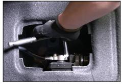
2. Open the battery access panel in trunk, on passenger side. Disconnect the negative battery cable with the 10mm socket and ratchet.
