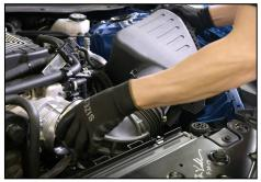
8. Gently remove the existing air induction housing and intake tube.
