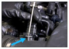
4. Locate the MAF sensor; remove the 2 screws with the T20 torx driver.
