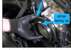
12. Connect the hump coupler to the throttle body with the arrow facing up. Make sure the side that has lettering is facing the throttle body and the clamp screws are accessible for tightening. Tighten only the clamp nearest the throttle body with the 8mm nut driver. Torque specs 5.1 +/-0.5Nm
