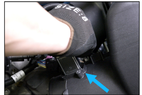
12. Gently pull the MAF sensor from its housing and set out of the way.
