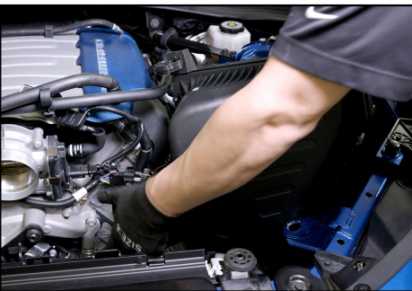
13. Gently remove the existing air induction housing and intake tube.
