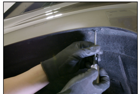
28. On Duramax Powered vehicles, maximum power is achieved by removing the air induction housing duct in the inner fender.
