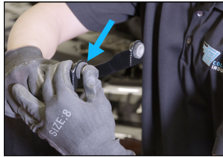
12. Reinstall the rubber grommets and metal standoffs from the factory air induction housing into the new air induction housing assembly legs.
