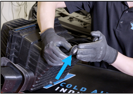
11. Remove the rubber grommets and metal standoffs from the factory air induction housing.
