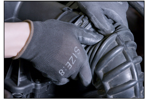
7. Remove engine cover duct from the factory air induction housing cover.
