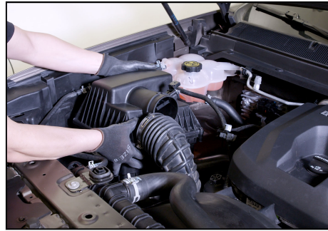
9. Remove housing from vehicle. Housing is held in by grommet in the wheelhouse. Pull firmly to remove air induction housing and rotate horn out of hole in fender.
