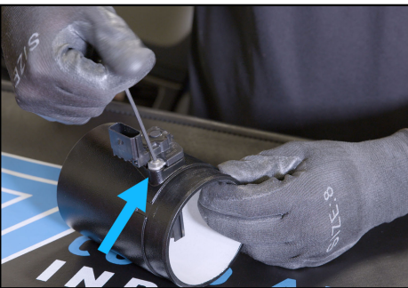
14. Place the MAF sensor into the MAF housing and reinstall the button head cap screws.
