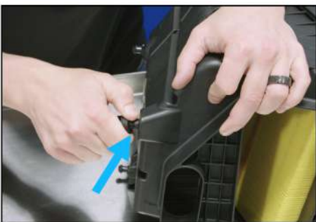
13. Remove rubber mounting pad.
