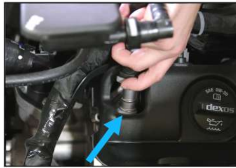
5. Unclip PCV fitting from valve cover.
