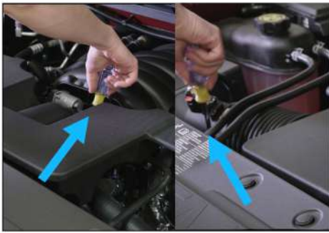
4. Loosen screws from CLEAN/AIR DUCT RESONATOR with 5/16 nut driver.
