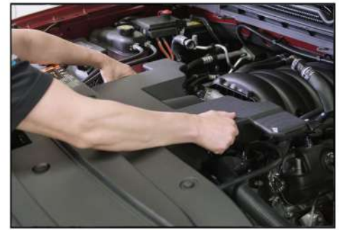
6. Remove CLEAN/AIR DUCT RESONATOR from vehicle.
