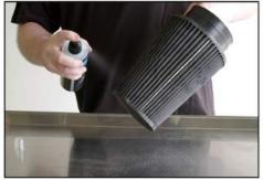
Liberally spray Cold Air Inductions Air Filter Cleaner on both sides of filter and allow to soak for 10 minutes to loosen the dirt. Do not allow cleaner to dry on air filter.
