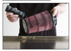
Apply Cold Air Inductions Air Filter Oil beginning an inch below the crown. Apply all the way around the filter. Continue to move down the filter and apply additional rings. NOTE: the rings should be approximately 2 inches apart. Stop when you are about an inch from the bottom of the filter. The oil will run down the filter and saturate the pleats.
