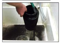
Rinse off air filter with cool low-pressure water from the inside out, in order to flush the dirt out of the filter. Continue to rinse the filter until all traces of cleaner are gone, and water runs clear through filter. It may be necessary to repeat steps 1 and 2.
