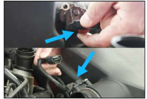
12. Disconnect MAF Sensor.
