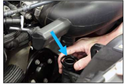
9. Disconnect sound enhancer tube.
