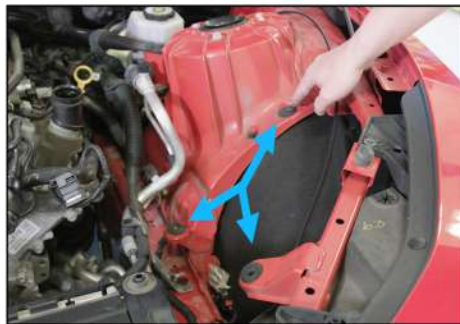
14. Reinstall any of the 3 OEM grommets that may have stayed attached to factory air induction housing assembly.
