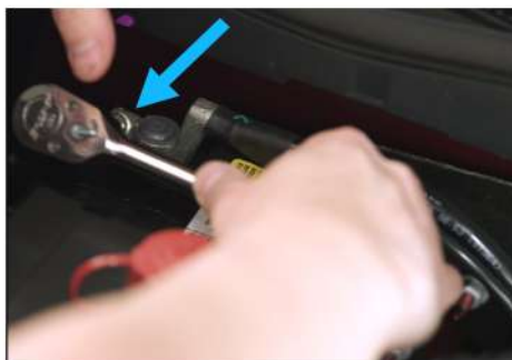
2. Disconnect the negative battery cable with the 10mm socket and ratchet.
