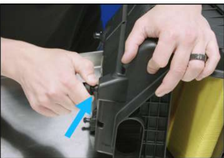
13. Remove rubber mounting pad.
