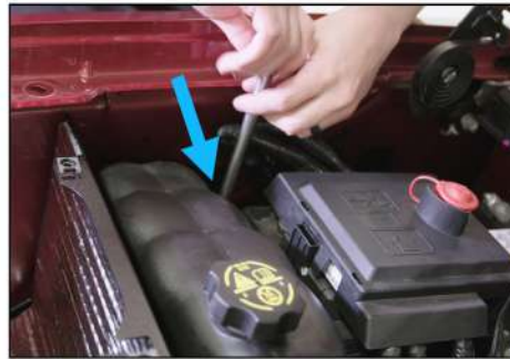
21. Reinstall the coolant reservoir.
