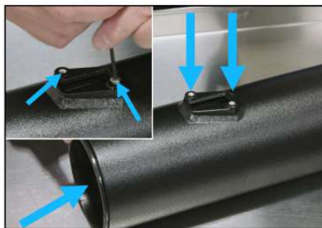
14. Remove BUTTON HEAD CAP SCREWS on the performance MAF/TUBE with 2.5mm allen wrench. 15. IMPORTANT Leave plastic insert inside of the tube and align holes where the MAF Sensor will be placed. NOTE: Do NOT install the filter prior to the MAF SENSOR. That would cause the insert to be misaligned with the MAF/TUBE.
