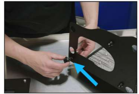
19. Install the factory rubber mounting pad onto the performance AIR INDUCTION HOUSING.
