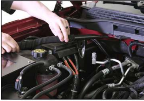
29. Reinstall the diagonal brace using the 13 mm socket and ratchet.
