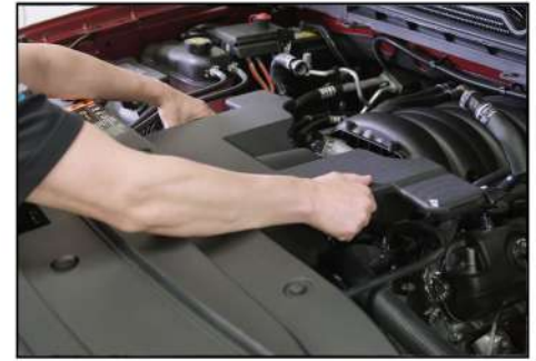
6. Remove CLEAN/AIR DUCT RESONATOR from vehicle.
