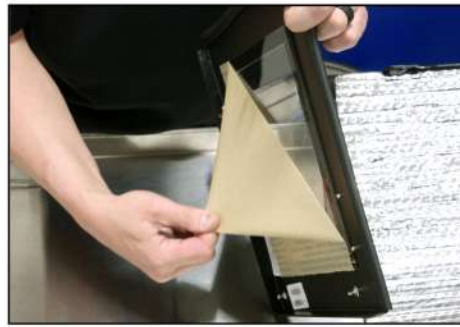
18. Remove the protective film over glass.
