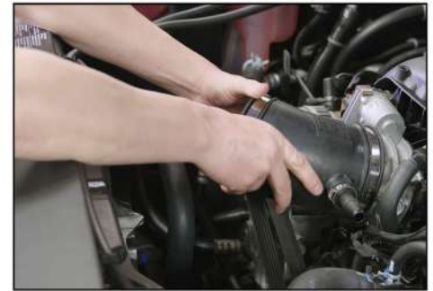
22. Install INLET/DUCT onto throttle body.
