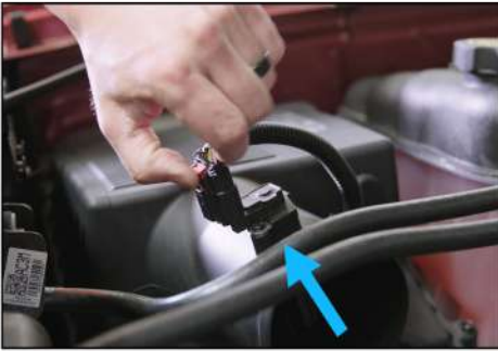
7. Gently disconnect the MAF sensor from its housing and set out of the way.
