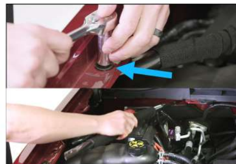
3. Remove diagonal brace using 13mm socket and ratchet.
