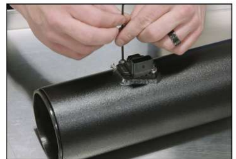
16. Install MAF sensor into performance MAF/TUBE, reinstall two BUTTON HEAD CAP SCREWS. Torque to 2.5 ft lbs.
