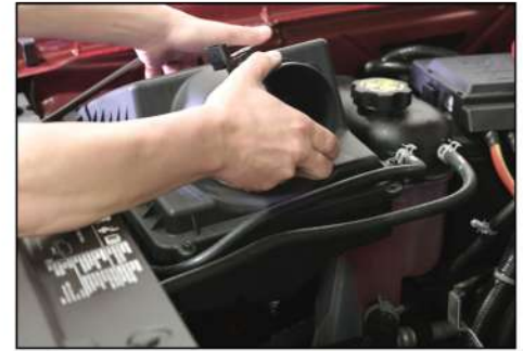
9. Remove OEM AIR INDUCTION HOUSING.
