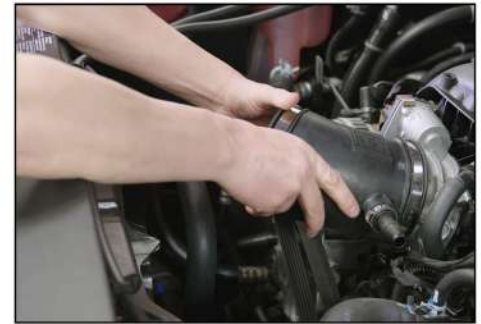
22. Install INLET/DUCT onto throttle body.
