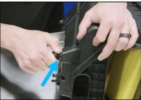
13. Remove rubber mounting pad.
