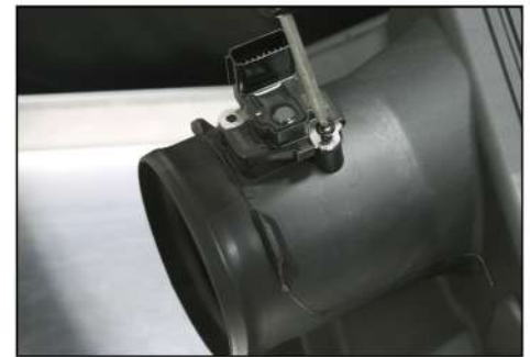
12. Place the factory AIR INDUCTION HOUSING on work bench. Remove the MAF SENSOR by removing the two screws holding it in place on the AIR INDUCTION HOUSING with the T10 torx driver. Take care not to damage the sensor as you will reinstall in the performance MAF/TUBE.
