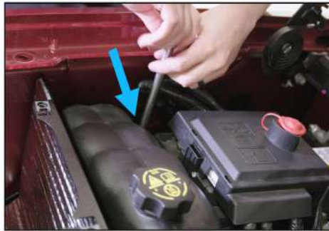
21. Reinstall the coolant reservoir.
