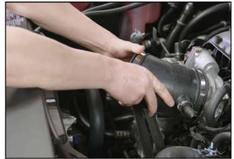
22. Install INLET/DUCT onto throttle body.
