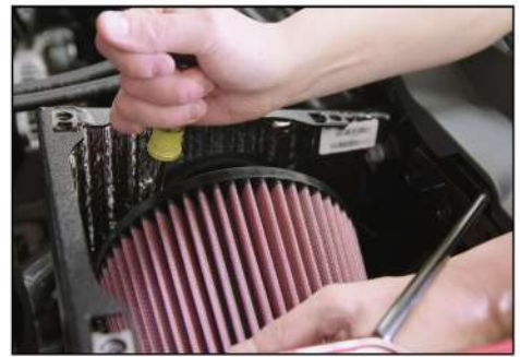
25. Insert FILTER ELEMENT onto MAF/TUBE. Tighten the clamp on FILTER ELEMENT with 5/16 nut driver.
