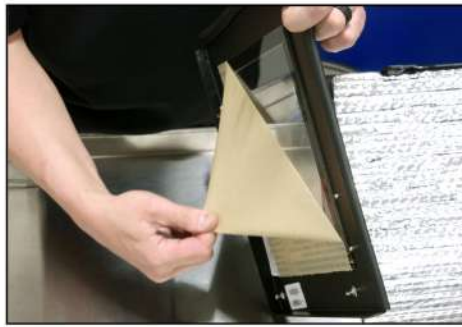
18. Remove the protective film over glass.
