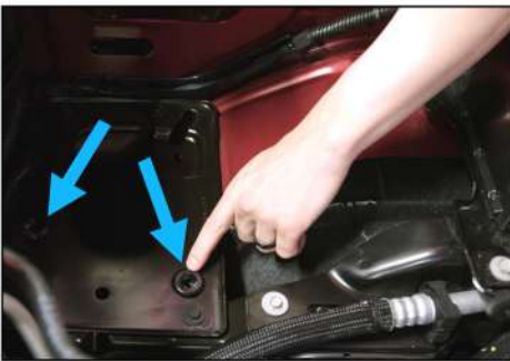
10. Make sure both grommets are intact in the grommet holes on the vehicle.
