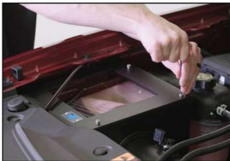
27. Attach the COVER to performance AIR INDUCTION HOUSING, using a 3mm allen wrench, gently push and turn the fasteners a quarter turn (only).
