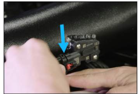
24. Reroute A/C wire under A/C hose and connect.
