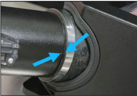
19. Align dot on MAF/TUBE to emboss on FILTER ELEMENT.
