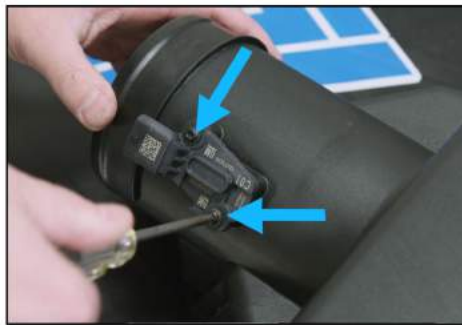
11. Remove the MAF sensor using a T20 torx by removing the two screws holding it in place on the MAF/TUBE. NOTE: Carefully handle the MAF sensor.
