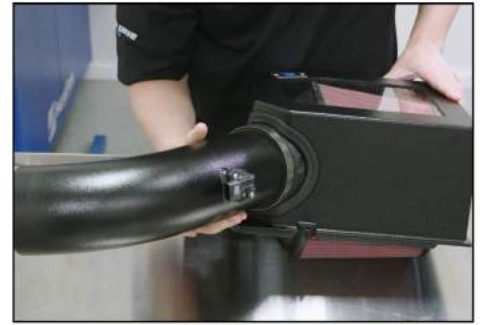
18. Install the MAF/TUBE into filter. Seat completely.
