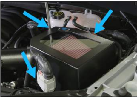
22. Replace the 3 screws into the AIR INDUCTION HOUSING, using the ratchet, 8mm socket and extension.
