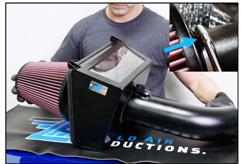
12. Insert the MAF/TUBE through the AIR INDUCTION HOUSING and into the high-performance FILTER ELEMENT. Tighten FILTER hose clamp with 8mm nut driver or flat head screwdriver to 53 lbf-in (6nm)
