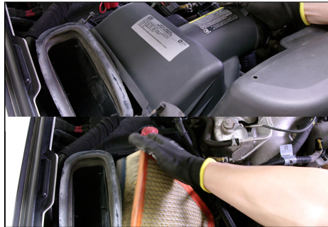
8. Remove the air induction cover and filter. Place the cover on a work bench.
