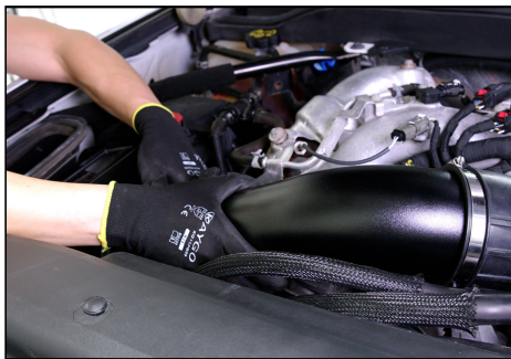
14. Install Air induction assembly onto OEM lower housing. Install MAF/TUBE into INLET/DUCT.
