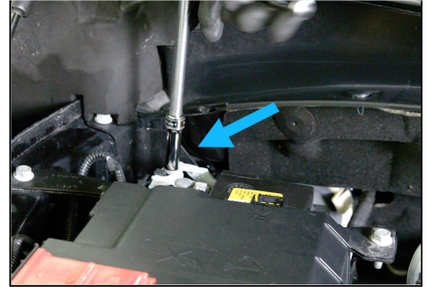
33. Reconnect negative battery cable using the 10mm socket.
