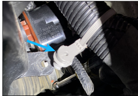
11. Remove the 4 wiring harness ties from Air Cleaner Outlet Duct.
