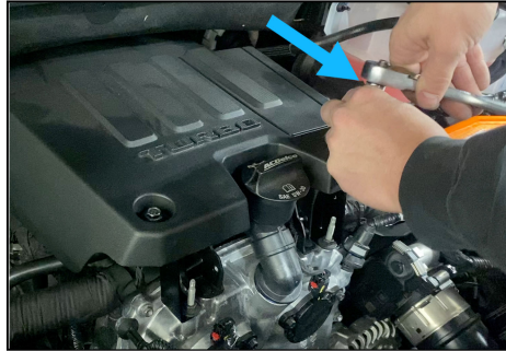
32. Replace engine cover onto provided brackets and tighten two bolts using the 8mm socket.
