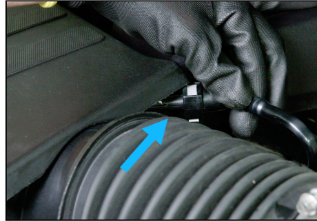
8. Remove (PCV) Fresh Air tube from Air Cleaner Outlet Duct.
