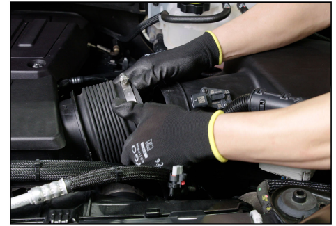
6. Disconnect outlet duct from induction cover.
