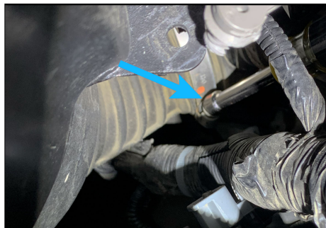
14. Using 7mm nut driver loosen hose clamp on Air Cleaner Outlet Duct near turbo inlet.
