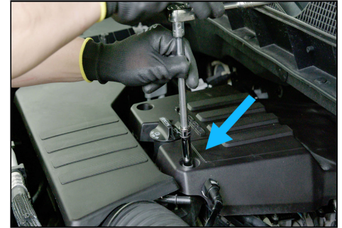
9. Using the 10mm socket remove the 2 bolts on engine cover. Then Remove engine cover.
